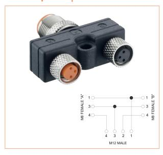
Passive actuator/sensor distribution box M8 Y-splitter, with two female M08 connectors, main connection: M12 male connector
