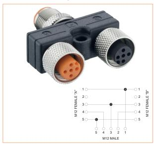
Passive actuator/sensor distribution box M12 Y-splitter, with two female M12 connectors. main connection: M12 male connector
