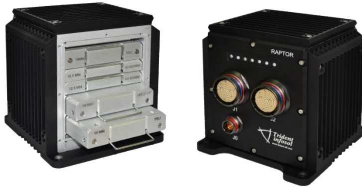
Figure 5: Trident infosal small-form-factor computers using VNX+ to meet the demands of harsh environments [7] (image courtesy Trident infosal).
